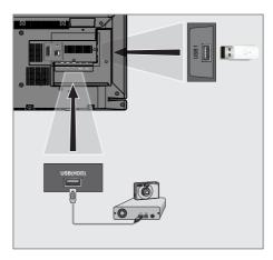
Connect the **USB(HDD)** USB interface on the television and the related data output on the external device (external hard disk, digital camera, card reader or MP3 player) with a USB cable;
