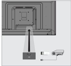
Plug the external hard disk to the USB(HDD) USB interface of the television; Notes:
