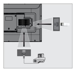
1 Connect the USB (HDD) interface of the television and the corresponding socket on the data device (external hard drive, digital camera, card reader or MP3 player) using a USB cable;
