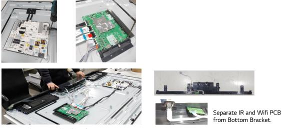
Remove the Bottom bracket after remove screw.
