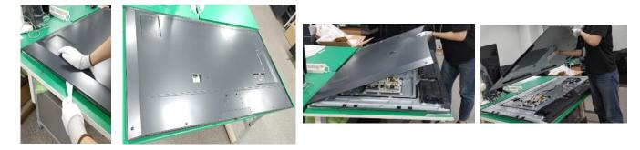
Once removed, this will expose the accessible electronic units (PCBs) which can now be easily removed with hand and screw driver.
