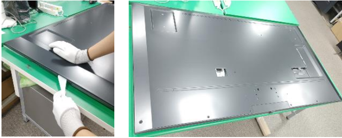
Remove the Back cover after remove screw.
