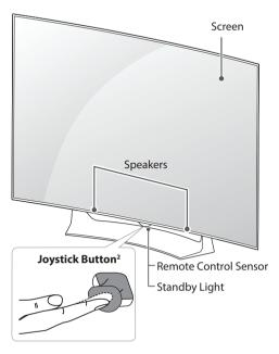
Screen Speakers Joystick Button<sup>2</sup> Remote Control Sensor Standby Light
