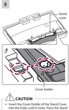
Insert the Cover Holder of the stand Cover into the holes until it clicks. Press the Stand Cover gently so that the non-woven fabric inside is attached tightly.
