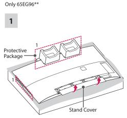
When assembling the stand, lay the front screen 1 Protective Package included in the product box on a table or product box and then place the TV screen face down on the Protective Package.
