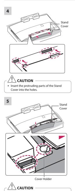
• Insert the Cover Holder of the Stand Cover into the holes until it clicks. Press the Stand Cover gently so that the non-woven fabric inside is attached tightly.
