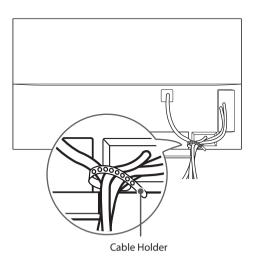
• Do not move the TV by holding the cable holder, as the cable holder may break, and injuries and damage to the TV may occur.
