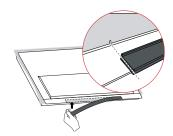
If you install the TV on a stand instead of mounting it on a wall, make sure that the removed brackets are reattached at the bottom of the TV. (Only OLED55/65E8\*)  Do not apply foreign substances (oils, lubricants, etc.) to the screw parts when assembling the product. (Doing so may damage the product.)
