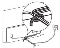
Attach the three covers when installing the wall mount. (Only when the item is provided.) (Only OLED55/65E9\*)
