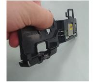
3. Disassemble Mechanical part (use screw driver)
