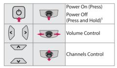
1 If the menu button is on the screen, pressing and holding the joystick button will let you exit the menu.
