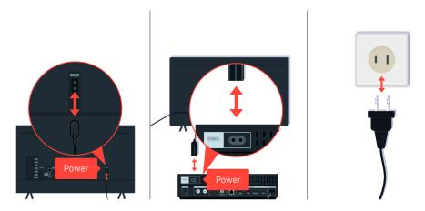
First disconnect and reconnect the power cables and HDMI cables on the back of your TV or the One Connect (OC) Box, then unplug the power cable and plug it back into the wall outlet.
