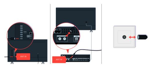
Check the antenna and input cable connections.
