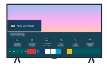
Check the volume on the screen. If a number for the TV volume is not displayed, select > Settings > Sound > Sound Output. Then, select TV Speaker.
