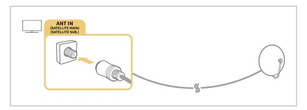
It is best to connect the both connectors using a Multi-Switch or DiSEqC Switch, etc and to set Aerial Connection Type to Dual.
