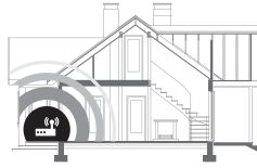
Unsuitable router position
