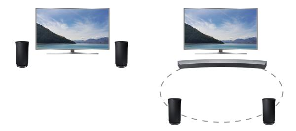
You can connect the TV to a Samsung wireless audio device through wireless network. At this time, two devices must be connected on the same network. For more information, refer to Wireless Speaker Manager ((a) > (a) Settings > Sound > Expert Settings > Wireless Speaker Manager).
