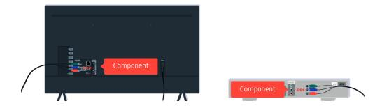
If a component cable is used, make sure that the coloured connectors are connected to the matching connectors on the external device and the TV.
