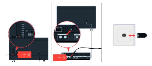
Check the antenna and input cable connections.
