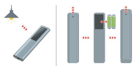
If you cannot see infrared signals, charge the remote control by using the solar cell or the USB port(C-type) on the bottom. If the remote control has batteries, replace them with new ones.
